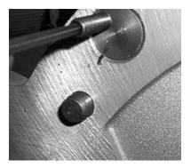
6. MARK THE PLATE FOR ANY ADDITIONAL TRIMMING OR CUTTING FOR CLEARANCE. IF THE PLATE WILL BE TRIMMED, BE CAREFUL NOT TO CUT TOO CLOSE TO ANY OF THE FASTENER HOLES AND REMOVE ANY BURRS LEFT FROM CUTTING.
