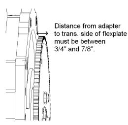
11. CHECK THE DISTANCE BETWEEN THE TRANSMISSION SIDE OF THE FLEXPLATE AND THE ADAPTER. THIS SHOULD BE BETWEEN .750" AND .875". **DO NOT PROCEED WITH THE INSTALLATION IF THIS IS NOT CORRECT.** ASSEMBLING THE MOTOR TO THE TRANSMISSION WITH THIS DIMENSION NOT IN TOLERANCE COULD RESULT IN TRANSMISSION OR STARTER DAMAGE. CONTACT WILCAP IF YOU FIND THIS DIMENSION TO BE GREATER THAN 7/8" OR LESS THAN <sup>3</sup>/4".
