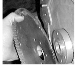
9. CAREFULLY ALIGN THE HUB SPACER/FLEX PLATE AND THE CRANKSHAFT BOLT HOLES WHILE PLACING THE HUB SPACER ONTO THE CRANKSHAFT. THE HUB SPACER SHOULD BE A CLOSE FIT TO THE
