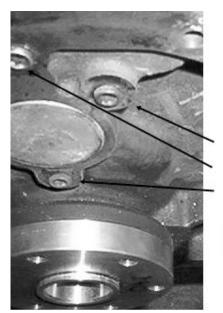
MAKE CERTAIIN THAT BLOCK PLUGS DON'T INTERFERE WITH ADAPTER PLATE DURING INSTALLATION!
