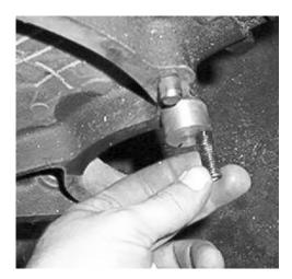
4. PLACE THE ADAPTER PLATE ONTO THE ENGINE BLOCK. IF NECESSARY USE A RUBBER MALLET TO FIT THE PLATE UP TO THE BLOCK FLUSH. DO NOT USE THE CAP SCREWS TO FORCE THE PLATE ONTO THE BLOCK. IF THE PLATE WILL NOT SIT FLUSH TO THE BLOCK, CHECK THE DOWEL PINS ON THE BLOCK TO SEE IF THEY HAVE BEEN DAMAGED AND MAKE CERTAIN THE BLOCK PLUGS ARE NOT INTERFERING WITH THE ADAPTER PLATE.
